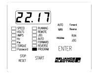
The display shows the time stamp, which is based on a 24-hour clock. Use the arrow keys to move between the day and time data.
